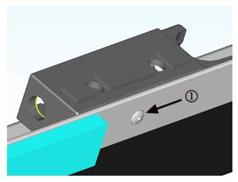
**5.** From the bottom side of the rail, use a 1/8 inch drill bit to drill out the old rivet (1).
