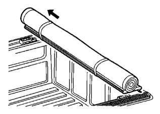
1. Remove the tonneau cover and the side rail(s) on the affected side. Refer to Soft Tonneau Cover Package Installation in SI.
