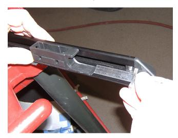
6. Reposition the pivot block 54.5 mm (2.15 in) from the end of the rail and re-secure the two set screws.
