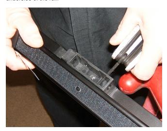
4. Loosen the two pivot block set screws securing the pivot block to the side channel of the rail assembly.
