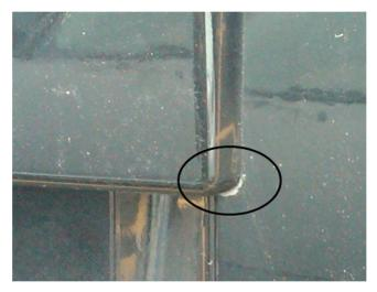
Some customers may comment on paint damage (shown circled above) on the liftgate at the lower outboard edges of the center applique.
