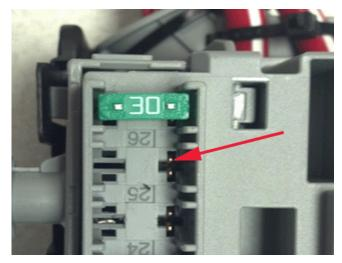
7. With the fuse removed, using the graphic above, determine which terminal is the feed side.
