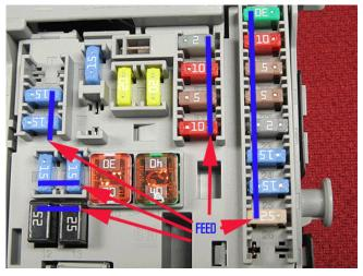
In the above graphic, the feed side of the fuse is highlighted in blue.
