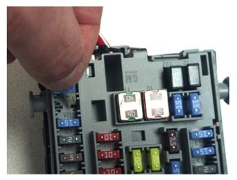
8. Using test adapter J-35616-35 for relay terminals, inserted in the feed side, perform a drag test and determine if the terminal has sufficient tension.
