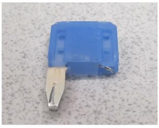
If J-35616-35 in not available, create a drag test fuse by cutting off one of the terminals as shown.
