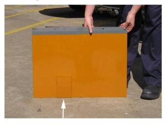
This first photograph shows a paint test panel finished in "Wildfire" metallic. The white arrow points to the paint "standard." This is the paint sample used to ensure color consistency.
