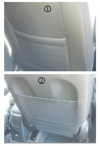
This occurs by design, with the driver non-folding seat (1) having a soft trim back cover and the passenger seat (2) having a hard plastic back trim for protective purposes, due to its ability to fold flat.
