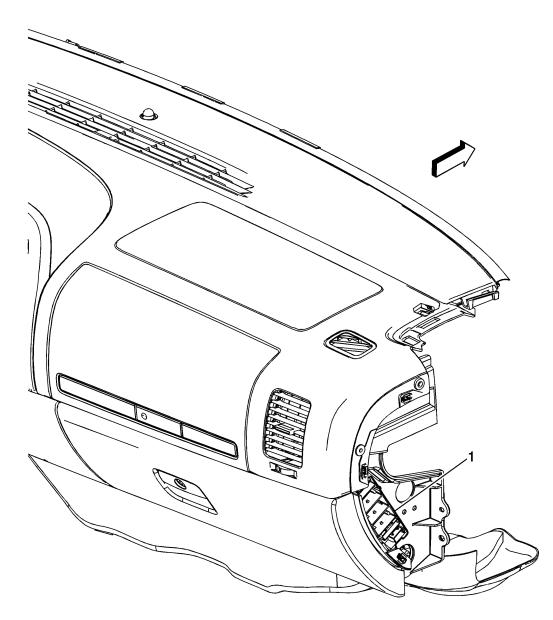
1. Remove the cover on the right side of the instrument panel, exposing the junction blocks.
