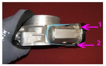
**9.** Turn over the throttle body and use a flathead screwdriver to remove the two clips (1, 2) as shown. Discard the clips.
