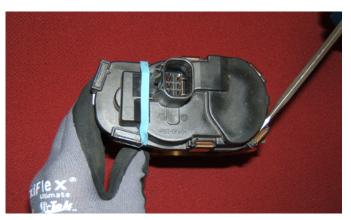
Notice: DO NOT PRY ON THE MACHINED SEALING SURFACE OF THE THROTTLE BODY INLET DUCT.
