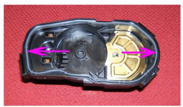
13. Verify that the TP sensor cover gasket HAS REMAINED in the TP sensor cover as shown. Ensure that the gasket is accounted for and remains with the old TP sensor cover.
