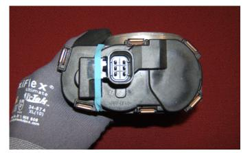
8. Secure a rubber band around the throttle body and TP sensor cover as shown.
