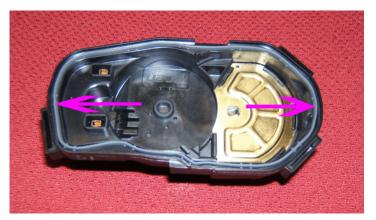
**17.** Verify that the TP sensor cover gasket is secure and properly positioned.
