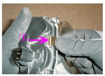
22. Install the first TP sensor cover clip (1) in the position shown.
