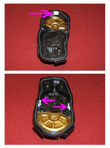
Notice: The three TP sensor cover alignment tabs are highlighted in white for identification purposes only.
