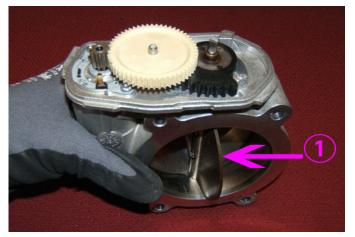
**20.** Rotate the throttle body plate to the WOT position (1).
