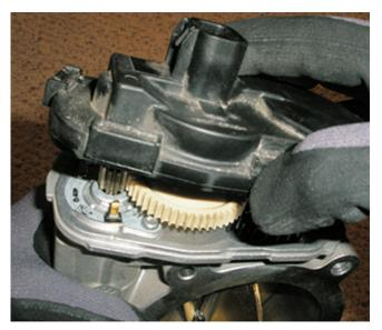
21. Position and install the TP sensor cover to the throttle body. Hold the TP sensor cover in position. If necessary for ease of the clip installation, secure a rubber band around the throttle body and TP sensor cover.
