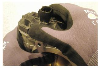
11. Hold the throttle body with your hand, so that the TP sensor cover is facing upward. Grasp the TP sensor cover and carefully lift it up and separate it from the throttle body.
