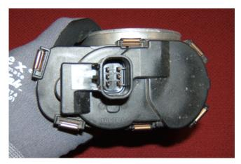
Notice: DO NOT mount the throttle body in a vise. The throttle body can be set on the top of a soft protected workbench area.
