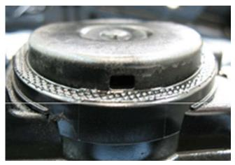
Note: The old style camshaft cover has a taller design PCV cap as shown in the illustration above.
