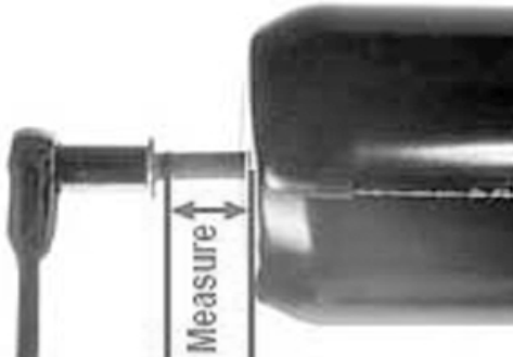
Figure 4. Integral Release Bolt Measurement
