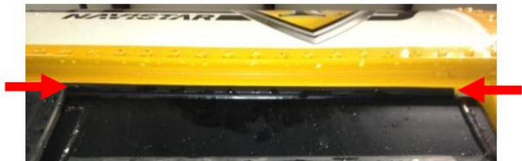
Upper Door Casing Seal Evenly Compressed
