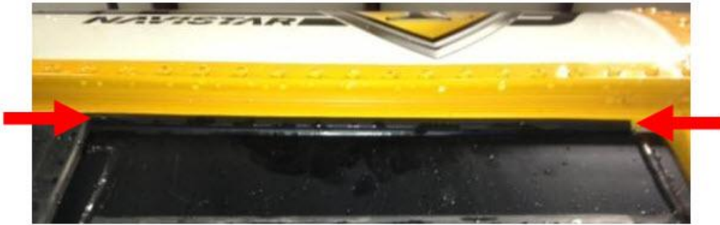
Upper Door Casing Seal Evenly Compressed
