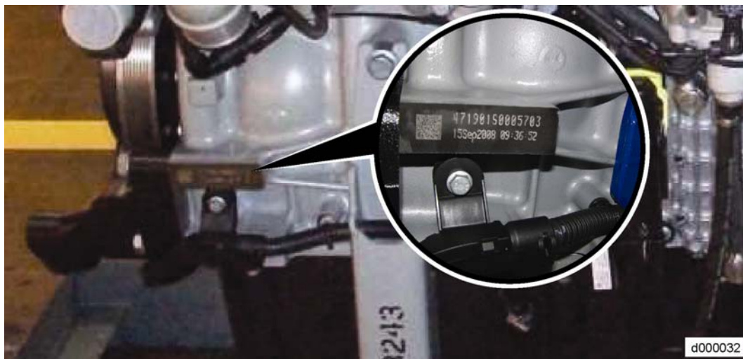
Figure 1- Engine Serial Number Location on Engine Block
