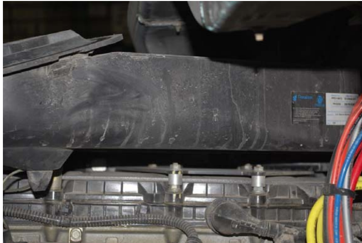
Figure 2 - Left Side Engine Air Filter Housing
