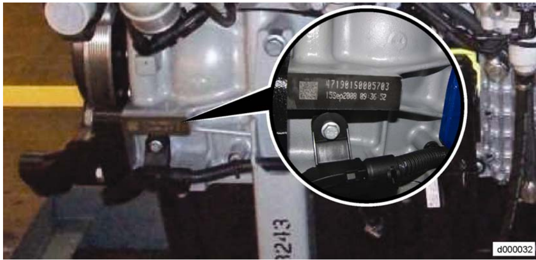
Figure 1- Engine Serial Number Location on Engine Block
