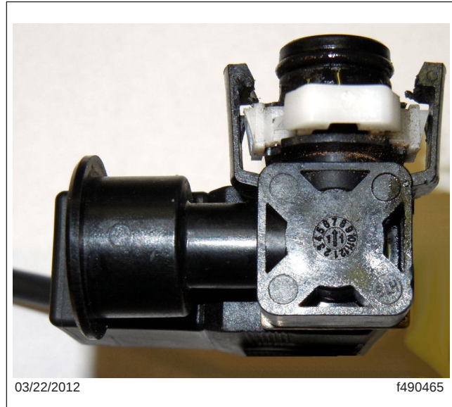
Fig. 2, 10-Watt Solenoid Valve ( 13.5 \pm 0.7 \Omega )
