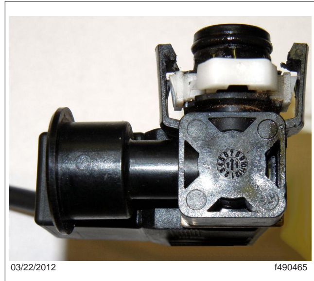
Fig. 2, 10-Watt Solenoid Valve ( 13.5\pm 0.7 \Omega )
