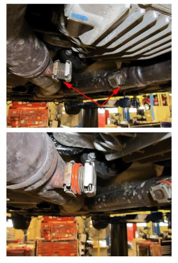
Technicians should follow the procedure below and install two silicone O-rings over each of the exhaust valve springs to dampen the rattle.
