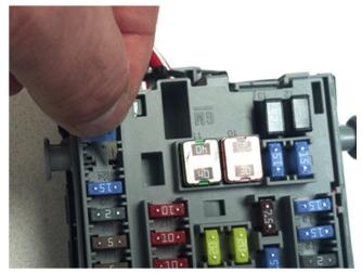
**8.** Using test adapter J-35616-35 for relay terminals, inserted in the feed side, perform a drag test and determine if the terminal has sufficient tension.
