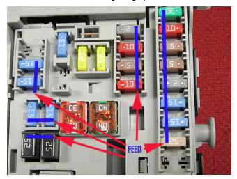
In the above graphic, the feed side of the fuse is highlighted in blue.
