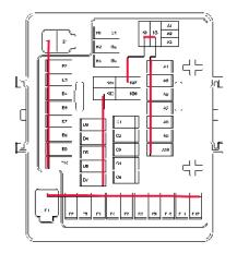
In the above graphic, the feed side of the fuse is highlighted in red.
