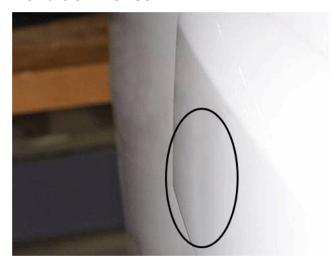
Some customers may comment on seeing a dimpling or deformation (shown circled above) near an outer edge of the liftgate center applique.
