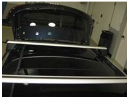
Figure 1. Roof carrier bars installed.
