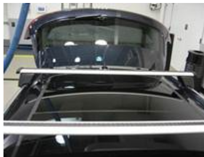
Figure 4. “Fluted” protection strips installed.
