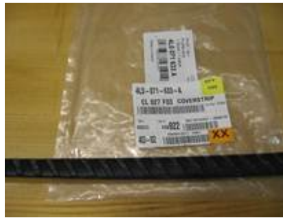
Figure 2. “Fluted” protection strips, part number 4L0 071 633 A.
