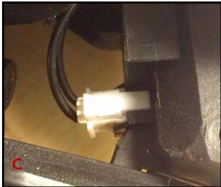
Figure 4. Connector “ C” shown in the locked position.
