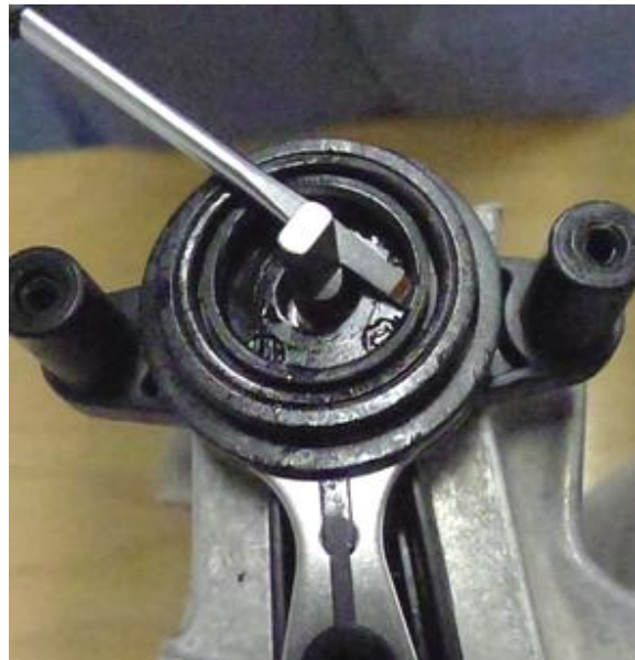
Figure 6. Removing seal ring.
