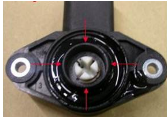
Figure 8. Lightly oiled sensor.
