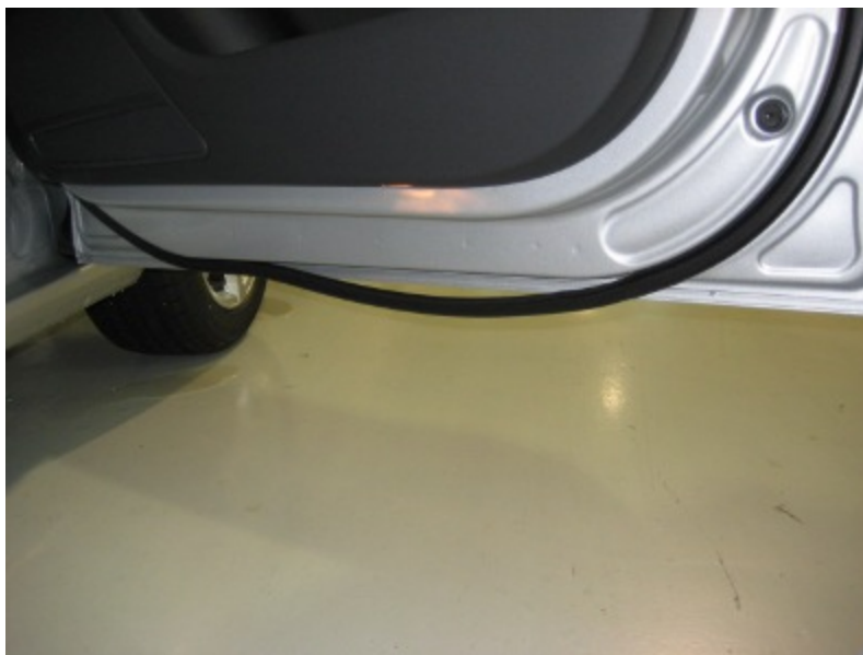
Figure 1. The outer door seal, partially detached.
