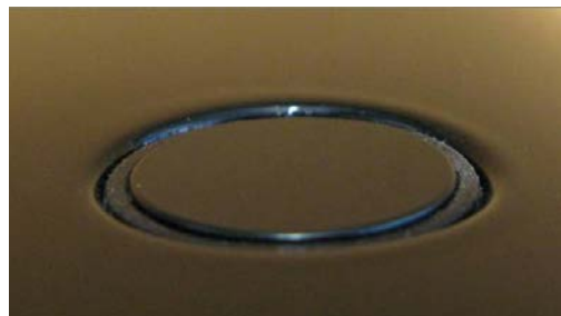
Figure 7. A correctly installed parking aid sensor.
