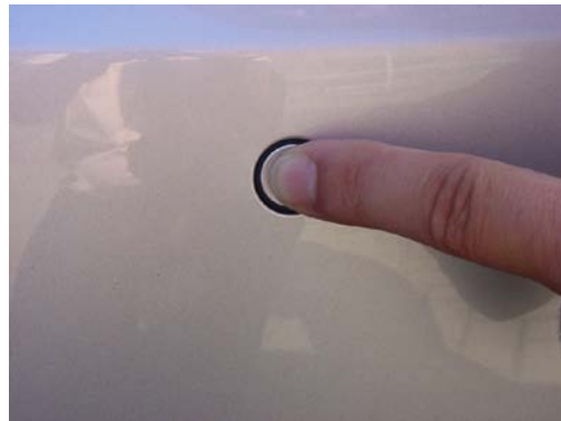
Figure 1. A pressure check on a parking aid sensor.
