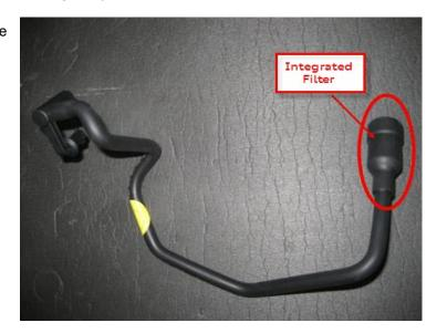
Figure 2. Ventilation Hose with Integrated Filter
