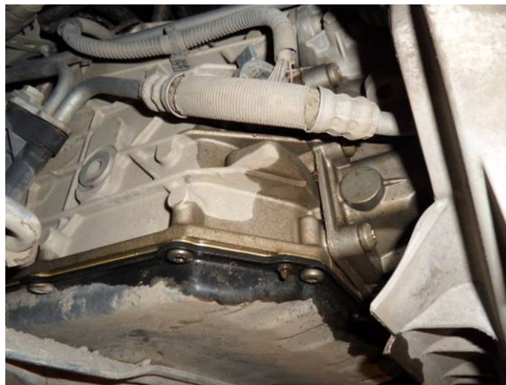
Figure 3. Leak between gearbox housing and intermediate housing.
