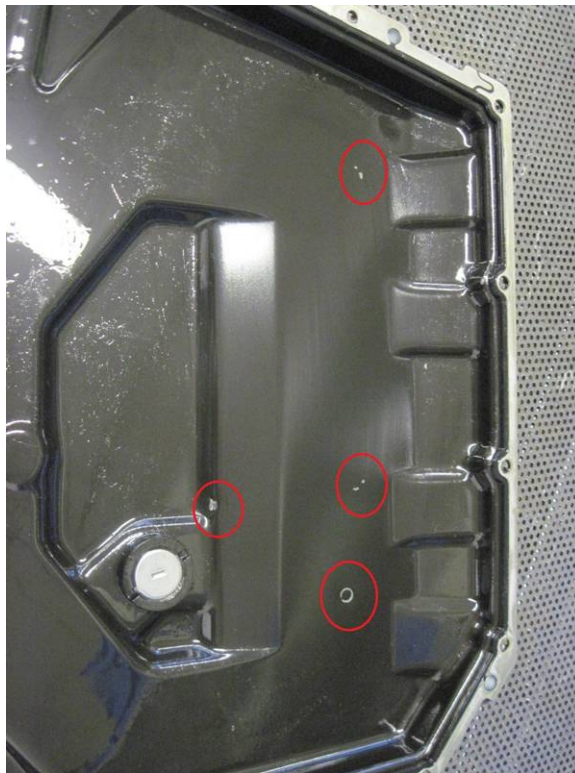
Figure 6. Damaged oil sump because of loose bolts.
