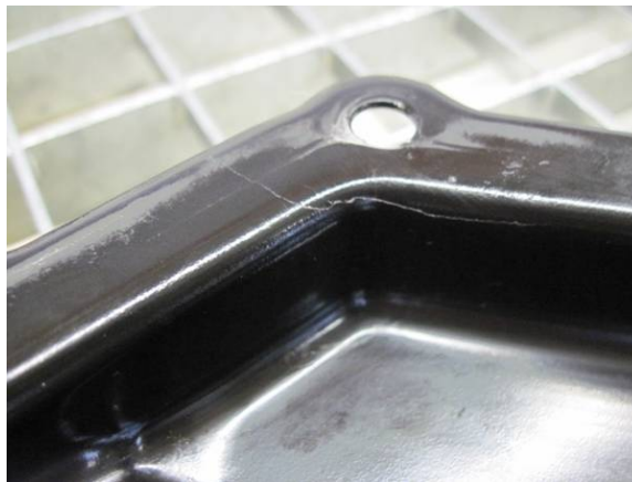
Figure 2. Crack in the oil pan.
