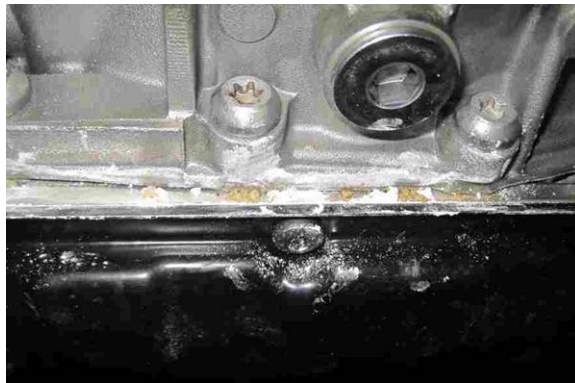
Figure 4. Leak located with Talcum spray.
