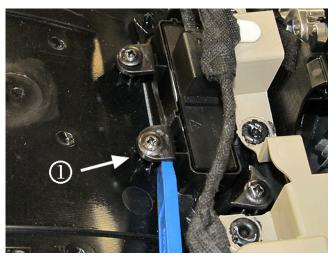
5. Using a trim stick, or equivalent, lightly pry against the standing boss (1) forcing the outer wall to move tight against the switch. Tighten the screw.
