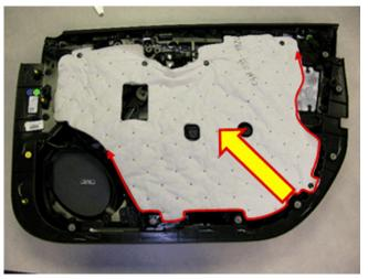
2. Peel back the sound absorber material from the trim panel enough to access the memory seat switch.
