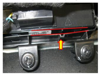
The cause of this condition may be insufficient retention of the seat switch snap features to the switch bracket.
