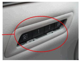
Some customers may comment that upon operating the driver seat memory seat switch buttons, the switch is pushing into the door trim panel.
