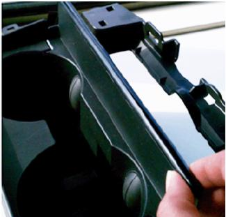
2. Pinch the two corners (as shown above) to ensure that the door is snapped together properly.
