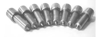
Aftermarket companies have developed a replacement performance/economy fuel injector nozzle. Refer to above illustration. The performance/economy fuel injector nozzles replace the OEM fuel injector nozzles. The aftermarket companies claim increased horsepower, improved fuel atomization, lower exhaust gas temperatures and increase fuel economy. This may cause additional fuel related driveability concerns and may cause internal engine damage to the pistons and fuel injector nozzles.
