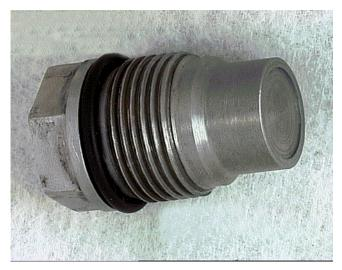
Aftermarket companies have developed a performance pressure relief fuel valve for Duramax<sup>™</sup> diesel engines. Refer to above graphic illustration. The performance pressure relief fuel valve attaches to the fuel rail in place of the OEM valve and will not allow any fuel return to the tank, giving 100% of the fuel to be available for additional engine performance. This may cause additional fuel related driveability concerns and may set the following DTCs:
