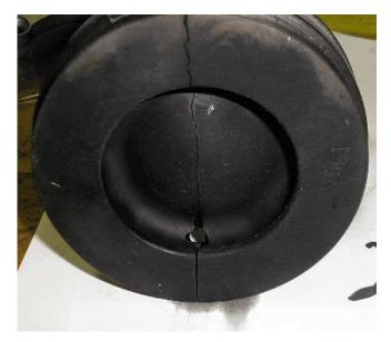
• Pistons will be cracked in the lip area, or a hole in the pistons.
