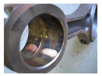
• Piston pin bore will show signs of scoring, the wrist pins will be discolored, and can have oil coking on them. The connecting rod bushing surface will have accelerated wear. The above illustration shows a connecting rod bushing.
