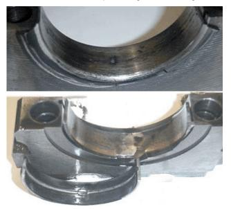
Bearing failure. Spun main bearings.
