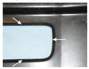
Clean the affected surface to remove any residual overspray of the backside protective paint. Apply \*Kent Automotive Acrysol, P/N 20005, or \*3M General Purpose Adhesive Cleaner, P/N 08984, or equivalent, to a clean shop towel and wipe the affected chrome surface.
