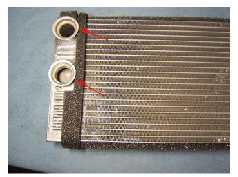
3. Install the new seal. Start at the pipe fittings as shown.
