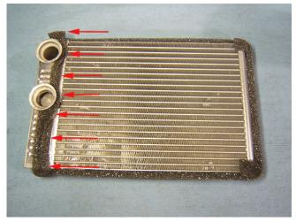
2. With the core on the bench, remove the foam seal on the tank end.
