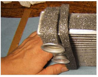
4. Wrap the foam seal around the tank end. Ensure the ends overlap as shown.
