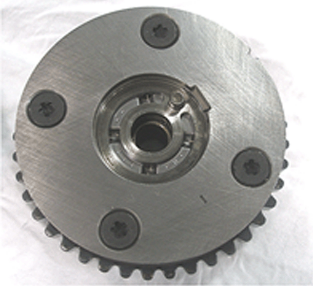
4 screw design uses P/N 12632859 thrust washer
