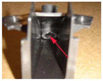
Ensure the hose does not become blocked by bottoming out squarely against the duct. Ensure it is positioned as shown. The duct is shown off of the vehicle with the foam seal removed to illustrate the correct hose position. This is not the installed position.
