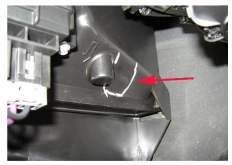
4. While holding the duct in position, use a paint pen to mark the heater case as shown, outlining the cooling duct.
