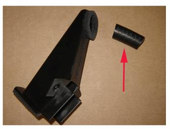
7. Cut a piece of 3/8 inch ID fuel hose to 25 mm (1 inch) in length.
