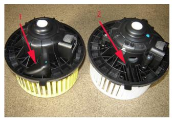
The design of the HVAC blower motor for these vehicles has been revised. The first design blower motor assembly has an integral cooling duct molded into the assembly (1). The second design blower motor assembly has a cooling port and uses a separate air duct that draws cooling air from the lower section of the HVAC housing assembly (2).
