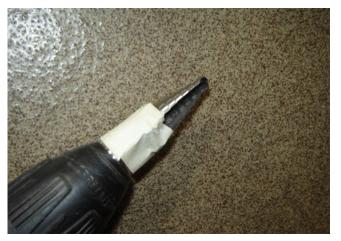
6. Using a single flute stepped drill bit, drill a 9/16-inch hole in the HVAC case lower half at the marked location. Do Not round-out the drilled hole.
