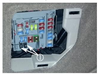
This action will remove power from the heated seat control module and reset the heated seat control module correcting the condition. While the initial cause of this concern is under review, the condition does not appear to return after the module is reset.
