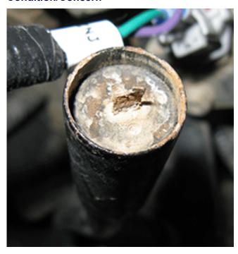
Some customers may comment that while attempting to remove the transmission fluid level indicator to check the fluid, the handle breaks off. Further investigation reveals that the metal indicator material was corroded and broke where the plastic handle is attached.
