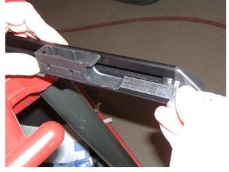
6. Reposition the pivot block 54.5 mm (2.15 in) from the end of the rail and re-secure the two set screws.
