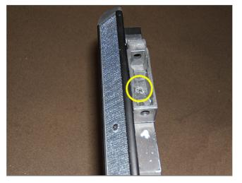
A rivet (location shown circled in the graphic above) that retains the pivot blocks to the side rail assembly may have loosened or detached.
