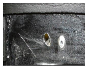
**Note:** A new hole is required for the rivet installation because the original hole may be distorted. For the front pivot block, drill the new hole forward of the original, and for the rear pivot block, drill the hole rearward of the original.
