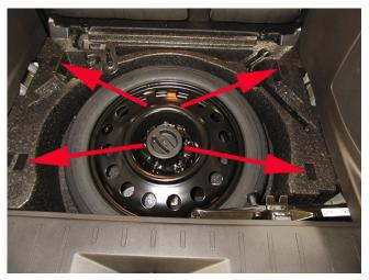
Some customers may comment the hook and loop type fasteners that secure the rear compartment load floor have separated from the molded plastic spare tire support assembly.
