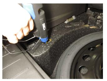
2. Using a hot glue gun, apply GM P/N 12377914 (in Canada, use 88864881) Hot Melt Adhesive Stick to the fastener mounting area on the spare tire support as shown.
