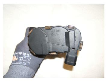
Notice: DO NOT mount the throttle body in a vise. The throttle body can be set on the top of a soft protected workbench area.
