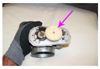
Notice: DO NOT allow the intermediate gear to fall out.
