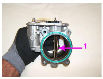
19. Rotate the throttle body plate to the WOT position (1).
