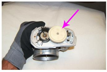
18. Grasp and hold the throttle body in the upward position. Lightly depress the intermediate gear to verify that it is fully seated and the gears are engaged.
