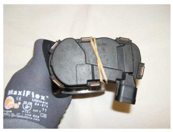
**8.** Secure a rubber band around the throttle body and TP sensor cover as shown.
