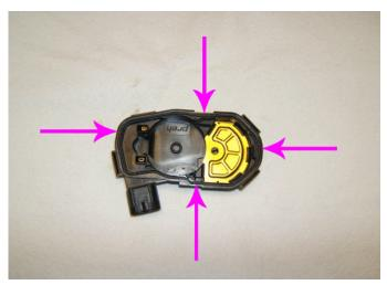
**12.** Inspect the TP sensor cover and verify that the TP sensor cover gasket **has remained** in the TP sensor cover as shown. Ensure that the gasket is accounted for and remains with the old TP sensor cover.
