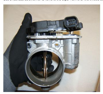
**10.** Hold the throttle body with your hand, so that the TP sensor cover is facing upward. Remove the rubber band securing the TP sensor cover. Grasp the TP sensor cover and carefully lift it **straight up** and separate it from the throttle body.
