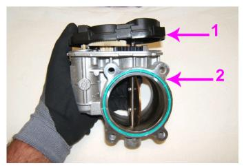
**20.** Position and **evenly** install the TP sensor cover (1) to the throttle body (2). Hold the TP sensor cover in position and for ease of the clip installation, secure a rubber band around the throttle body and TP sensor cover.
