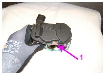
21. Install the first TP sensor cover clip (1) in the position shown.
