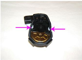
Notice: The three TP sensor cover alignment tabs are highlighted in white for identification purposes only.
