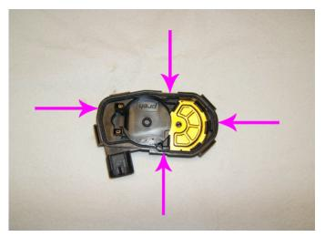
**16.** Verify that the TP sensor cover gasket is secure and properly positioned.
