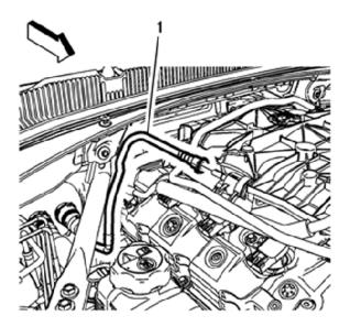
1. Inspect the evaporative emission hose/pipe for contact.
