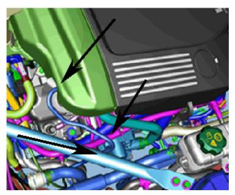
2. If contact is found between the evaporative emission hose/pipe and the engine cover, battery cable or diagonal brace, install a 435mm (17 in) piece of flexible conduit over the nylon portion of the evaporative emission hose/pipe.
