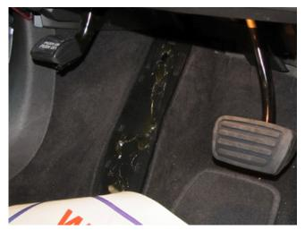
4. Using a heat gun, carefully apply five nickel size pools of hot melt to the carpet base. Apply quickly to help minimize the glue running down the base.
