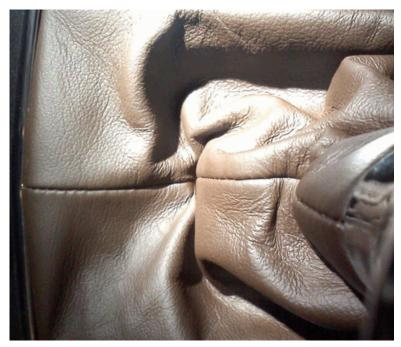
Inspect the shifter boot for signs of being pinched. See the picture above, which shows the pinched shifter boot condition. If you find a pinched shifter boot, please request the following new shifter boot through the warranty parts center. Attached below is a form to use to order the shifter boot from the WPC. There are four different color shifter boots; see the chart below for the proper WPC part number for the color shifter boot that is needed.
