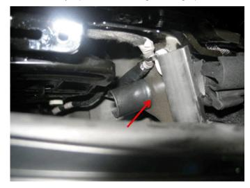
**Important:** It is normal for the quarter glass window to make light contact with this drain when the window is rolled down. Modifications to the upper lip of the drain can be made if cycling the window results in the drain tube being pushed out of the sheet metal. An opening on the top of the drain tube that resembles th opening on the bottom of the tube can be made for this condition. The drain will not fall out of the body sheet metal unless the drain is not fully seated.
