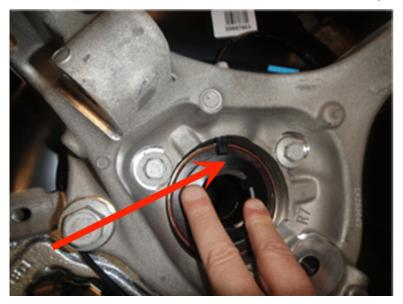
Original washer has a larger diameter and, if off-center, may contact the WSS.
