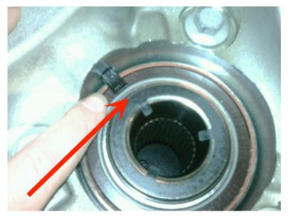
Replacement washer has a smaller diameter.
