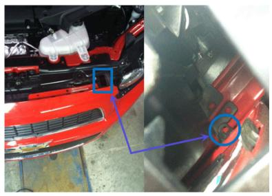
If no concerns are found with the baffle, proceed with using chassis ears on various components and locations of the vehicle to help isolate the area of the concern.
