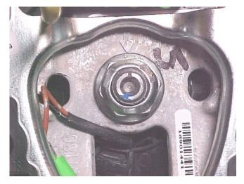
If the steering wheel and shaft marks are not properly aligned, remove the steering wheel and align the steering wheel to the shaft. Inspect to make sure the splines are properly engaged and install the steering wheel nut and torque to factory spec per SI. Perform a toe adjustment.
