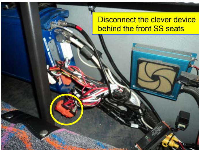
Disconnect E modules behind the SS light panels
