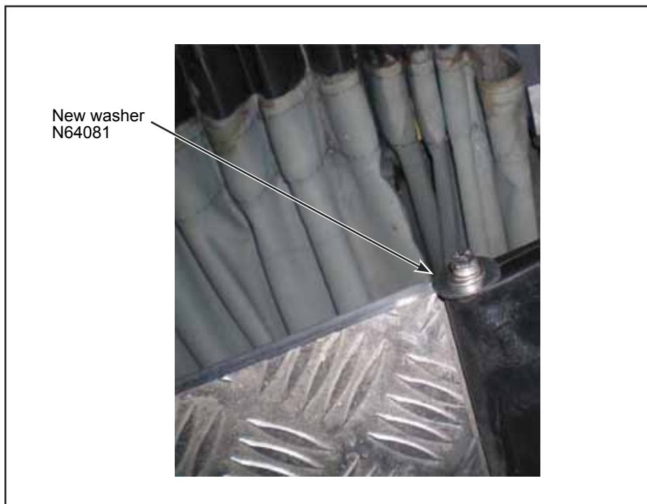
Figure 4 - New Washer Installation
