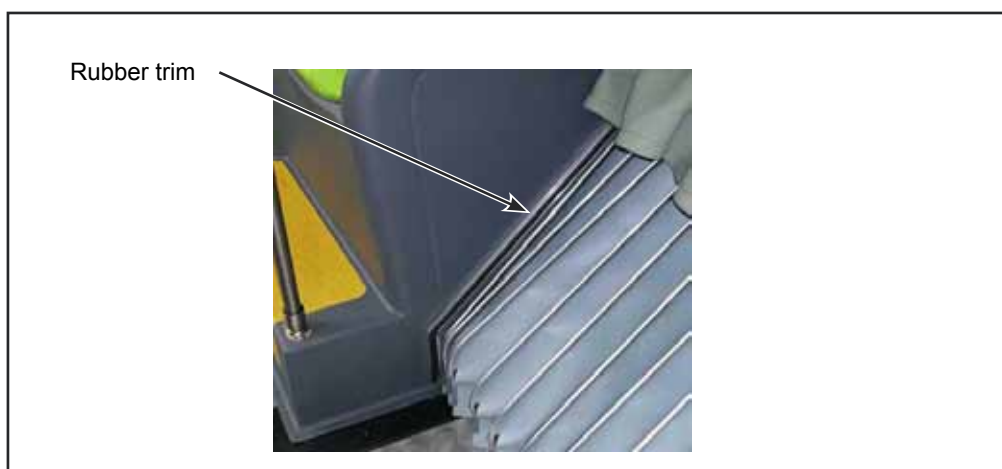
Figure 5 - Rubber Trim Installation
