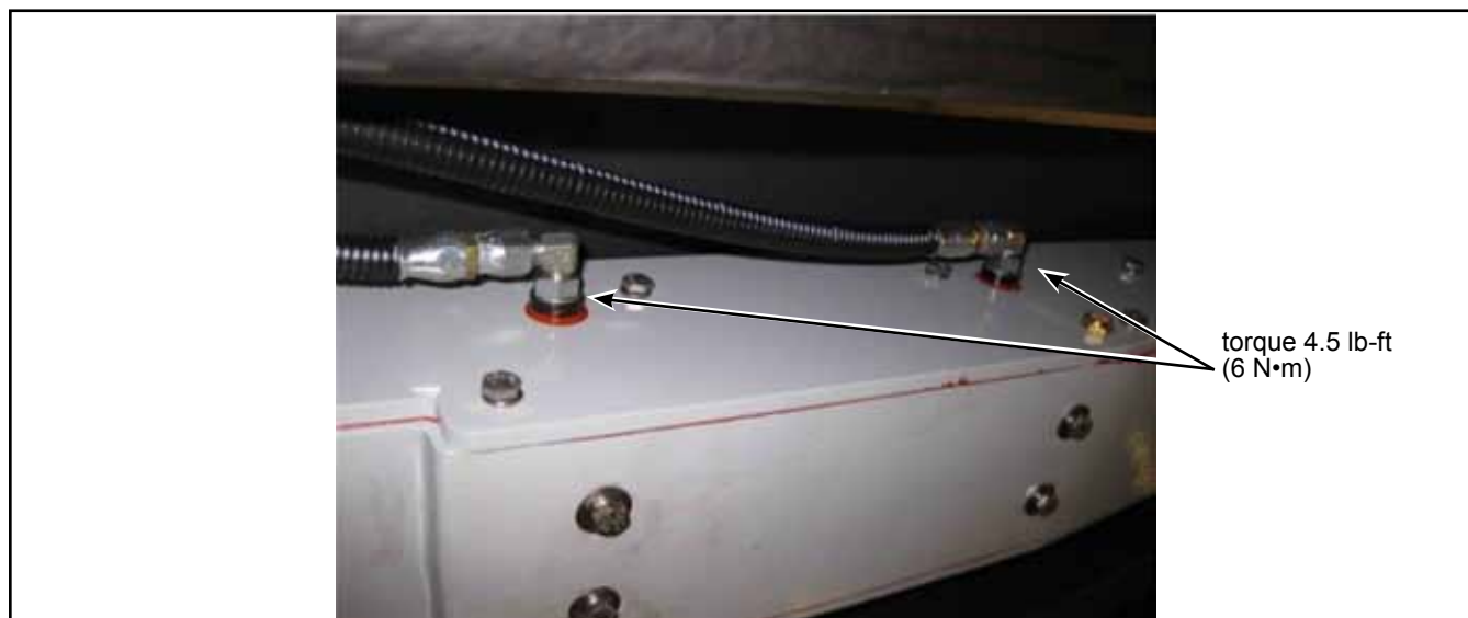
Figure 9 - Hydraulic Connector Torque
