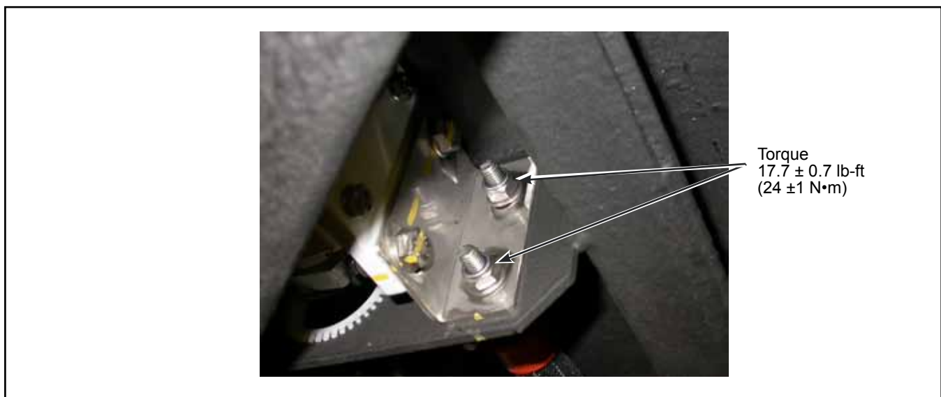
Figure 8 - Bolt Torque
