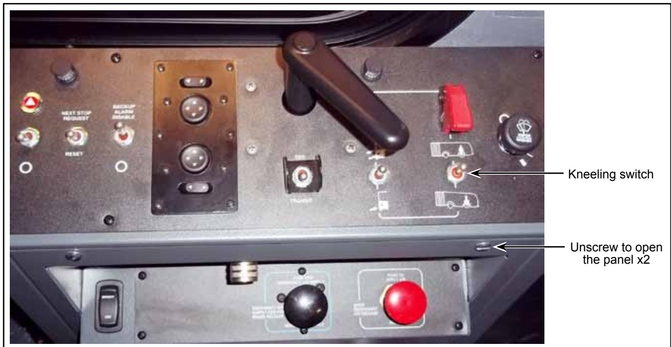
Figure 1 - Overhead View of the Lateral Console
