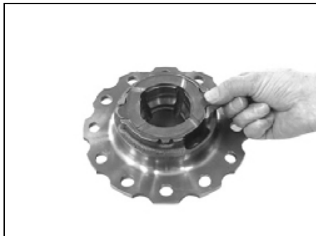
Figure 17 - Thrust Washer Placed in Differential Cover Carrier
