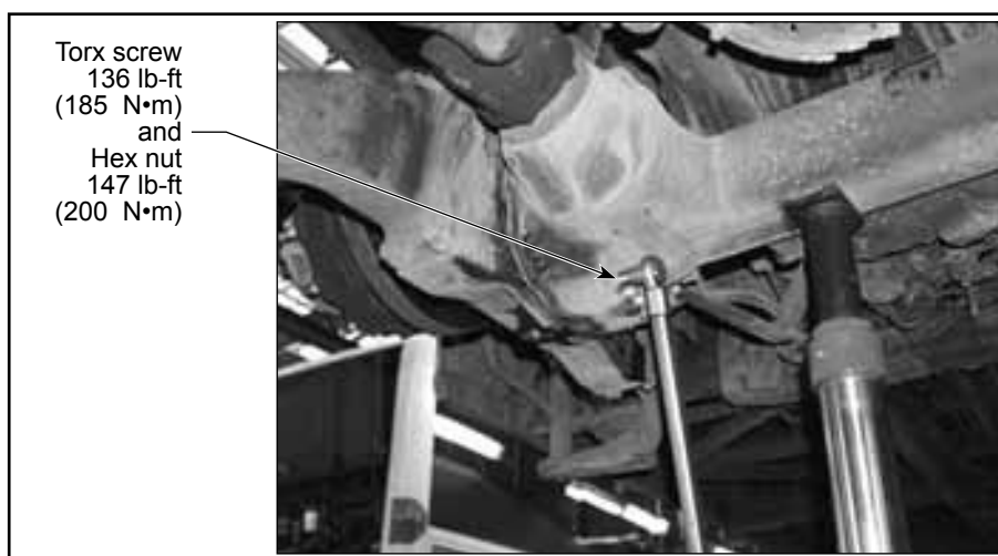
Figure 21 - Portal Drive Mounting
