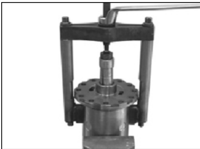
Figure 12 - Differential Cover Removal
