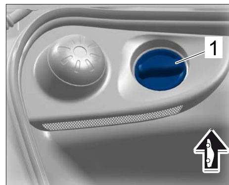
Cap on coolant filler neck in luggage compartment
