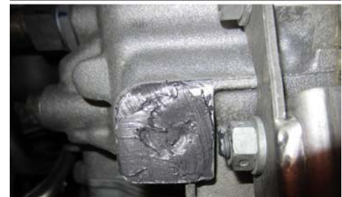
Applying sealing compound
