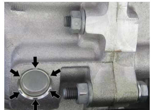
Existing staking marks on crankcase
